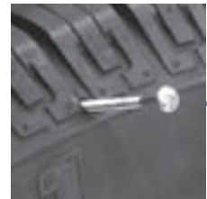
Puncture - Normally, the only evidence of a puncture will be a cut that extends from the tread of the tire through the inner liner.
