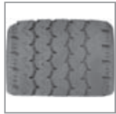
Rapid Shoulder Wear
