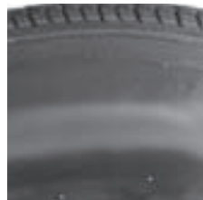
Under-Inflated Tire - An abrasion may run around the circumference of the tire and wrinkles may be observed in the inner liner.
