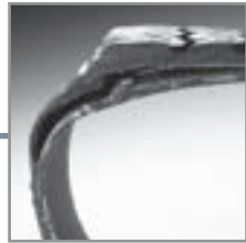
Sidewall Bubble - A bulge that appears on the outside of a tire is usually a sign of separation.
